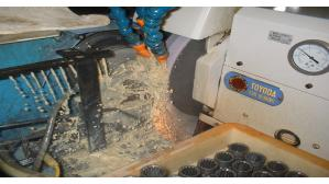
We have 7 I.D. grinders which we can grind from .500 up to 12" internal diameter, 6 through feed and plunge centerless grinders that can grind up to 5" diameter and up to 20 inches in length through feed. 2 double disc grinders that can grind .050 and up thickness, 3 manual surface grinders and a Blanchard grinder with a
